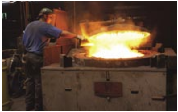
Skillets are baked at over 600° F before passing through the Larkin cooling system which reduces skillet temperatures to a safe-to-handle 85° F.
